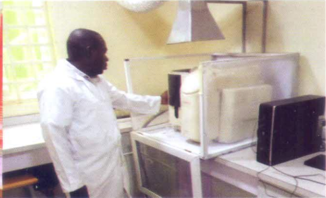
Atomic Absorption Spectrophotometry (AAS) Used for trace metals analysis
