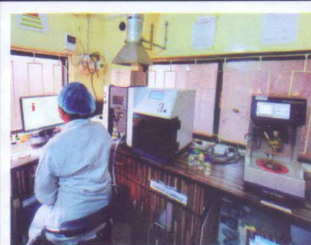
Testing of Trace & Heavy metals with AAS & Testing of engine oil with Flash point.
